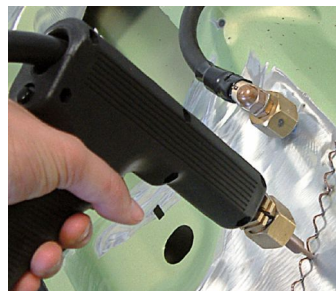
Corrugated wire spot welding
